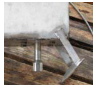
Fig. 2: SPRn 4115 L 2T and welded faceplate to ensure that sensor is submerged in liquid, stainless steel box with handle for easy removal from manhole
