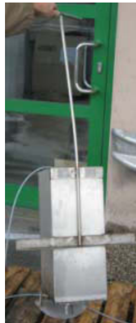
Fig. 2: SPRn 4115 L 2T and welded faceplate to ensure that sensor is submerged in liquid, stainless steel box with handle for easy removal from manhole
